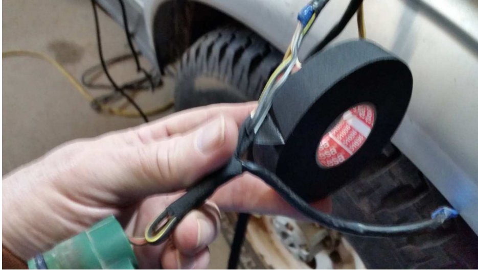
Double wrap at junctions with branches of wires.
