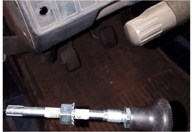
Remove nut and thread thru hole
