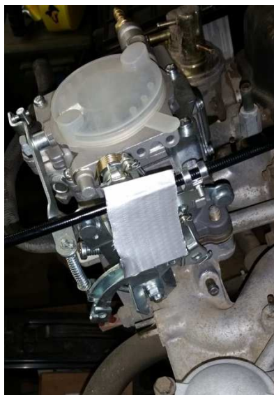
Mark where to cut housing Here tape is used to mark
