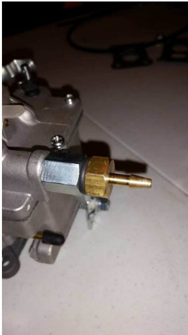
Fuel Barb Installed
