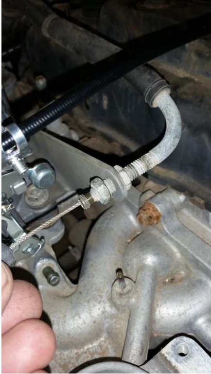
Mount Throttle cable and Bracket
