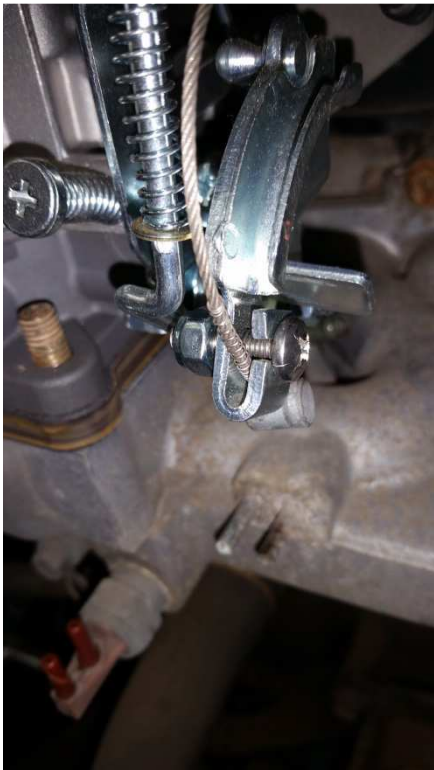
Install Bolt and Lock Nut as shown
