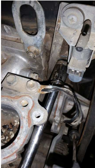
Remove Solenoid Bracket
