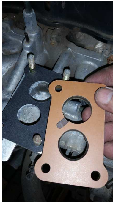
Insulator installed as shown
