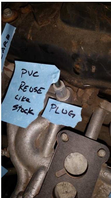
Vacuum Ports Identified
