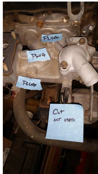
Vacuum Ports Identified
