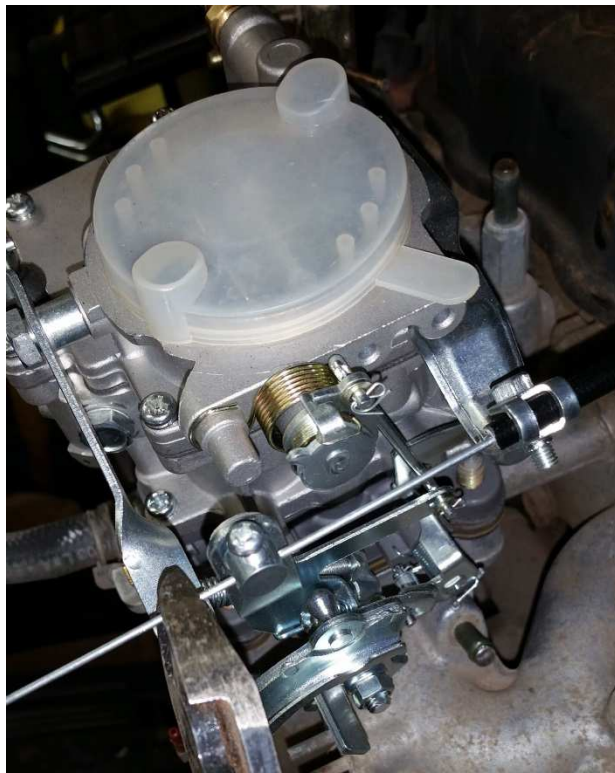
Trim off excess choke wire/cable
