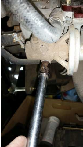
2 bolts on EGR removed
