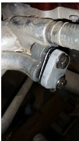
Gasket and Cover in place
