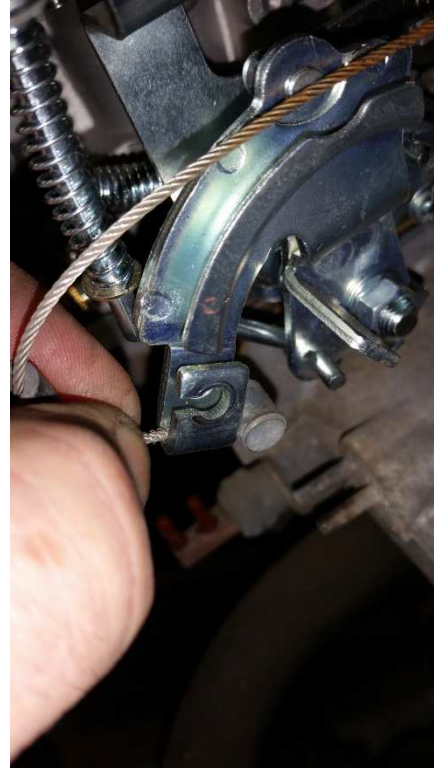
Locate Cable end as shown
