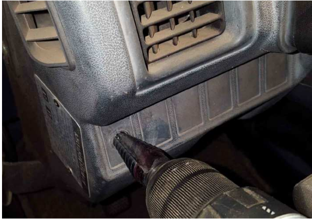
Step drill hole for Choke Cable
