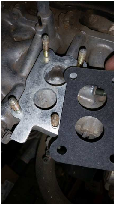
Manifold Gasket goes on first - Larger Hole towards Head
