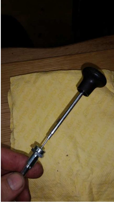
Pull inner cable out of housing
