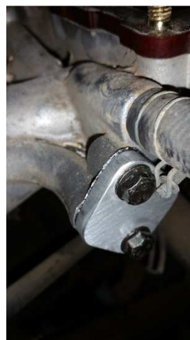
Block Off Plate tightened
